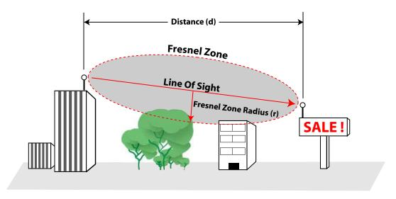
The size of the Fresnel Zone is determined by the transceiver's frequency and by the distance between the antennas:
