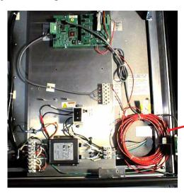
Serial I/O cable and TEMP/SYNC cable
