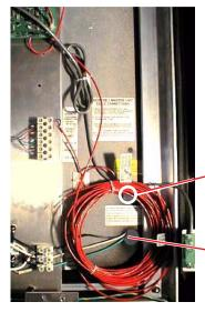
NOTE: Do *not* route the Serial I/O and TEMP/SYNC cables with the power wires.
