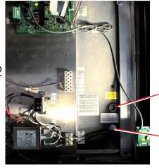
NOTE: Do *not* route the Serial I/O and TEMP/SYNC cables with the power wires.
